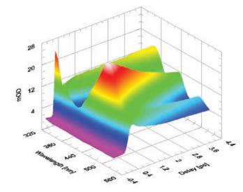
3D graph (left) and and Representtive transient spectra (right) of DDBBE organic dye dissolved in acetonitrile taken with FemtoFrame II. Excitation with 0.2 uJ, 1kHz, 346 nm pulses from the doubled output of Rainbow 20F. Temporal range -0.2 ps (dark blue) to 5 ps (red).
