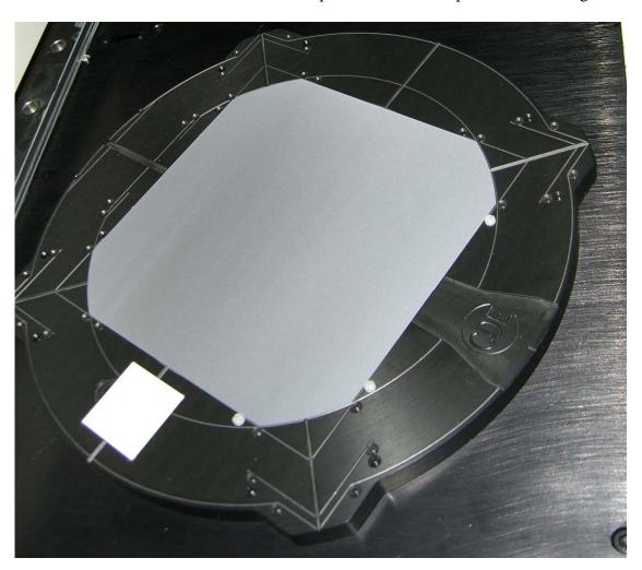
We measured all these samples using a 6 x 6 grid pattern with 10mm edge exclusion. Since the edges of these samples are rounded, the 4 corner sites are outside the 10mm edge exclusion and re automatically removed by the pattern generator.
