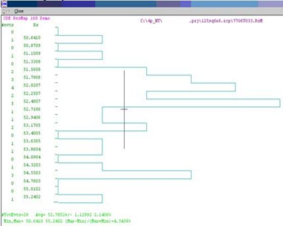
2.1.4 Wafer data plot, labels the data value on each site. The '+' labels data with values above the average; the '-' labels data with values below the average; the 'x' labels bad and immeasurable data; and the 'o' labels data rejected by Sigma rejection, in this case it is set at  $3\sigma$ .
